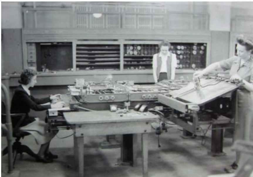
Kay McNulty, Alyse Snyder, and Sis Stump operate the differential analyser in the basement of the Moore School of Electrical Engineering, University of Pennsylvania, Philadelphia, Pennsylvania, circa 1942–1945 http://en.wikipedia.org/wiki/Kathleen_Antonelli
